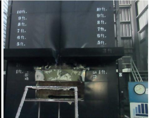
**Picture 3:** The exterior face of the test specimen at the end of the 10:00 minutes observation period after 30:00 minutes of fire propagation test
